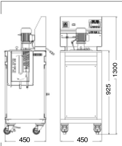
The TB300M bath is an instrument used to calibrate transducers, RTD and temperature-measuring sensors in the field and in the laboratory. The possibility to generate positive and negative temperature ramps makes it suitable for use in calibrating and testing thermostats.
