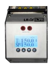
Thanks to the many available inserts, the calibrators can be adapted to the calibration of temperature probes of most common diameters (see page 3).
