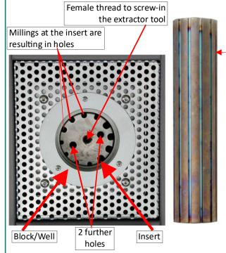
Inner diameter of the metal dry block: 60 mm diameter x 275 mm depth.
