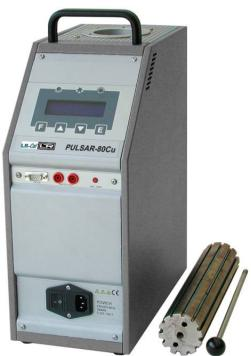
The temperature calibrator LR-Cal PULSAR-80Cu consists of a metal block diameter 80 mm x length 300 mm, heated by a resistance which winds around the outer surface of the block. A hole with diameter 60 mm and depth 275 mm is made in the block for the appropriate reduction inserts.
