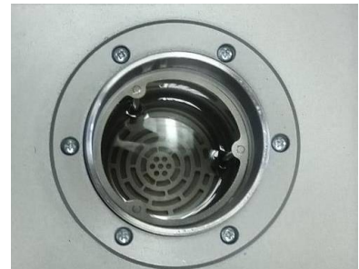
Top view: Calibration bath opening with basket and mixer rod
