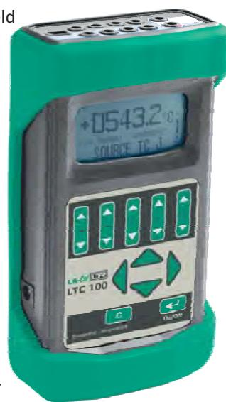
The Temperature Calibrator **LR-Cal LTC 100** simultaneously measures and sources ten types of thermocouples and seven resistance temperature detectors (RTD), whilst automatically capturing the calibration results. It measures millamps whilst sourcing or simulating millivolts, TCs, RTDs or ohms to calibrate transmitters.
