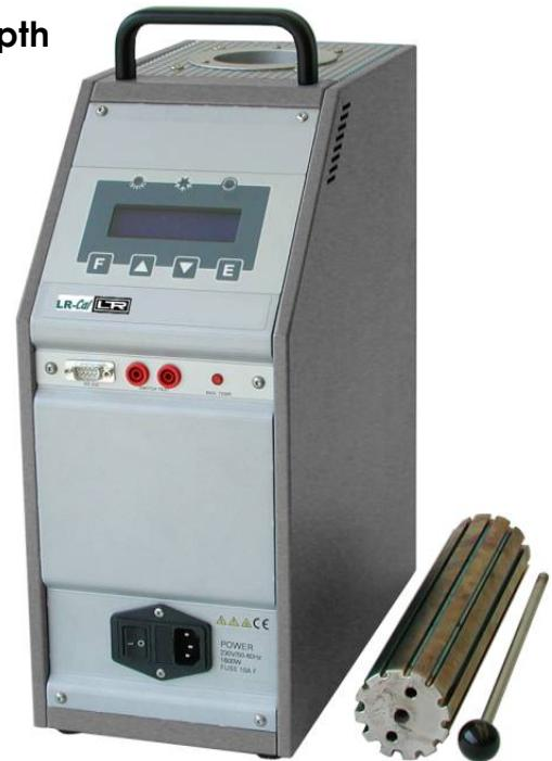
The LR-Cal LTC-DB-0550-60 is equipped with a counter-current forced air cooling system, which keeps the temperature in the upper part of the well low. This system enables to check even very short probes, without heating the connection head or the handgrip. The calibrator is equipped with a PID microprocessor controller with a resolution up to 0.01°C, setting of the standard of measurement in °C, °F and K, programming of ascent/descent ramps and storage of a thermostats' operative temperature.
