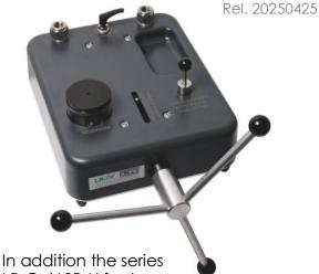
LR-Cal LSP-H feature a threaded spindle which only runs within the pump body. Thus there is no adverse bending moment acting on an outstanding spindle, and particularly for field use this has the advantage that the dimension of these pressure comparison pumps will not change when the spindle is turned during operation. The series LR-Cal LSP-H needs only little force to generate also high pressures.
