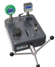
The pressure comparison test pumps models LR-Cal LSP-H are equipped with strainer dirt collectors in the pressure ports as well as in the bottom of the operation fluid reservoir. This reduces considerable the risk of material pollution of the operation fluid.
