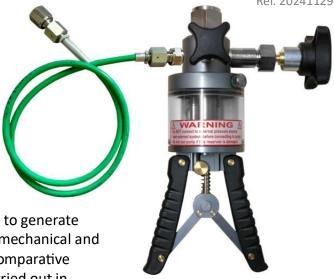
The Pressure Test Pump LR-Cal LPP 1000 is used to generate pressure for checking, adjusting and calibrating mechanical and electronic pressure measuring instruments by comparative measurements. These pressure tests may be carried out in laboratories, workshops or directly on-site at the measuring point.
