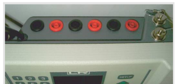
Image: Electrical ports at the LR-Cal LPC 300
