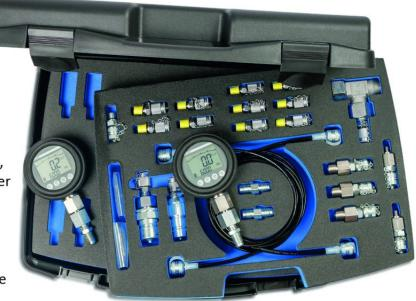
The HPKD-AH hydraulic test case has been specially designed to meet the requirements for checking and testing the hydraulic systems on universal commercial vehicles (e.g. Unimog) as well as agricultural and construction machinery.
