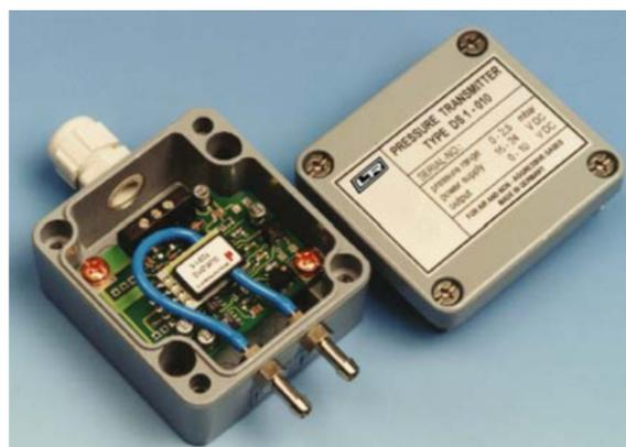
The pressure transmitter models **DS1** and **DS2** measure differential pressure, gauge pressure or vacuum, optional velocity of flow. The measured values are transmitted to voltage (0...10 V) or current (4...20 A), optional as frequency signal (0...10 kHz). The version with current output (4...20 mA) is realised in two wire technic.
