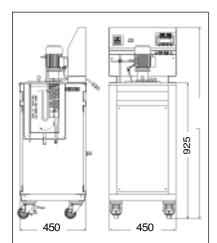
The BK40M bath is an instrument used to calibrate transducers, RTD and temperature-measuring sensors in the field and in the laboratory. The possibility to generate positive and negative temperature ramps makes it suitable for use in calibrating and testing thermostats.
