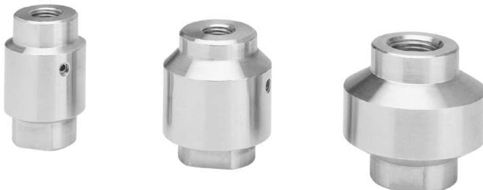
Diaphragm seals are designed to isolate the sensing element of pressure gauges and pressure switches from process fluids that may be corrosive, viscous, sedimentous and / or with a high temperature. The diaphragm is welded to the body, to ensure separation of the filling fluid from the process medium. The threaded connection make it easy to use on all applications where the reduced size of the system is important and also where gauges of 63 mm. diameter are required.
