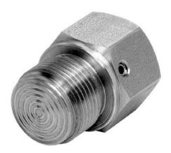
Diaphragm seals are designed to isolate the sensing element of pressure gauges DS 63 and electronic transmitter from process fluids which may be corrosive, viscous, sedimentous and/or with a high temperature. The diaphragm is welded to the top housing and leak proof tested, to guarantee a separation between process fluid and fill transmission fluid. This construction feature and its compact design suits many application that require frequent maintenance.
