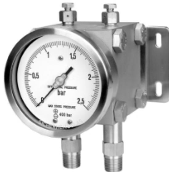
These instruments are used to check filter obstructions, pressure drops, flow rate differences, level, measurements and generally the difference between two pressures of equal or different circuits. The measuring element is formed by two diaphragms, acting on the same movement. In this way the pointer senses only the difference between the two pressures corresponding respectively to upstream and downstream circuit pressure.
