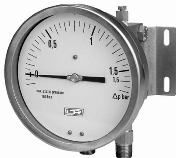
These instruments are used to check filter obstructions, pressure drops, flow rate differences, level, measurements and generally the difference between two pressures of equal or different circuits. The measuring element is formed by two diaphragms, acting on the same movement. In this way the pointer senses only the difference between the two pressures corresponding respectively to upstream and downstream circuit pressure.
