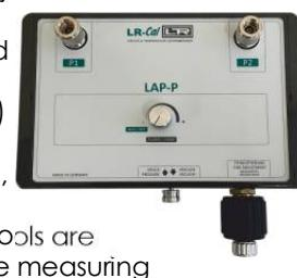
Both the test specimen and the reference pressure gauge (pressure calibrator) are mounted on top of the electric test pressure pump, using suitable thread adapters if necessary. No tools are required for connecting the measuring instruments, hand-tightening the instruments is quite sufficient.
