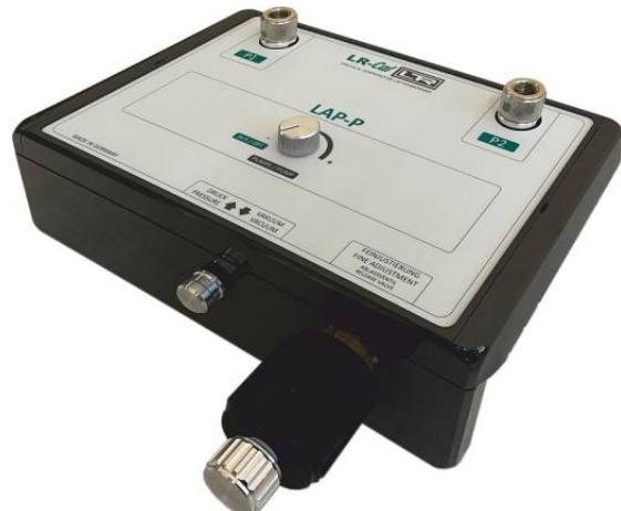
The LR-Cal LAP-P electric calibration pressure test pump is used for simple pressure generation, without manual effort, for checking, adjusting and calibrating mechanical and electronic pressure measuring instruments by comparative measurements.
