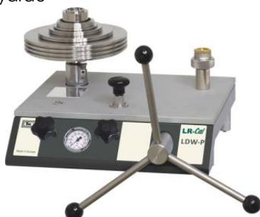
**Dead weight tester** (Pressure balances) are working on a basic physical principle ( $P = F/A$ ). They include a manual pressure source. A recertification every five years is adequate for deadweight tester.
