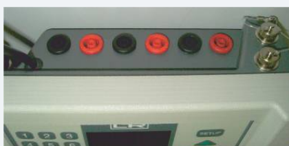
Elektrische Anschlüsse des LR-Cal LPC 300 Electrical connections
