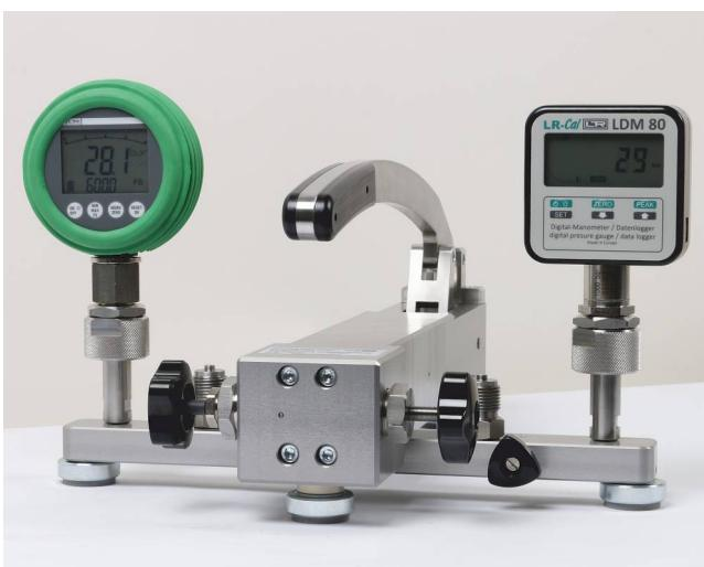
The pneumatic pressure comparators LR-Cal LPP 60-T and LR-Cal LPP 140-P enable very easy generation of calibration pressure up to 60 bar (870 psi) resp. 140 bar (2030 psi), switchable to vacuum generation -0.95 bar (-28 inHg). Via the sensible volume adjustment valve it is possible to adjust the test pressure very sensitive. The adjustable pressure relief valve allows easy calibration at „decreasing pressure“.
