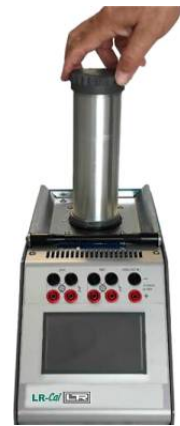
(3) Screw the lid completely shut and insert the insert into the calibrator.
