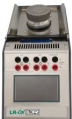
(4) Once the insert is in place, unscrew the cap and proceed with calibration.
