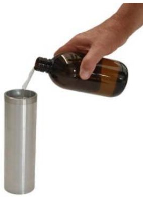
(2) Fill with calibration fluid to a level 3 cm below the upper edge.
