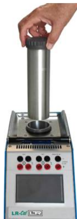
(5) If a change of calibration fluid becomes necessary, pull the insert out by hand.
