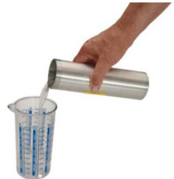
(6) Drain the calibration fluid, clean the insert with paper towels, and fill with the desired calibration fluid.
