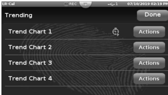
This menu item allows to make graphs of the analogue inputs and outputs. To start this trending view, you must press one of the buttons „Actions“, as four different graphics can be displayed, but not simultaneous.
