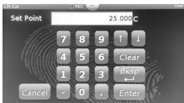
Instrument version with external reference probe: The set point (SP) can only be modified on screen page 1 (PT100 Int), regardless if the equipment is controlled by internal or external probe.
