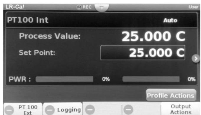
If you have the optional instrument version, you can tip on the arrow on the right, which allows to go to the second page. „PT100 Ext“ is displayed.
