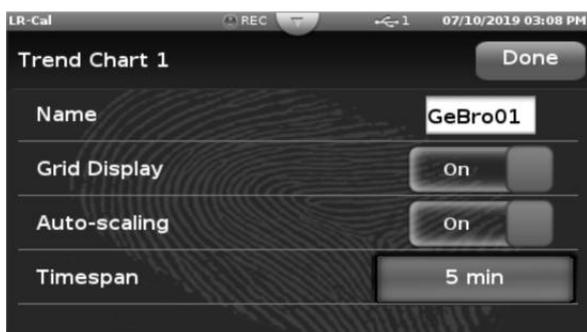
**View / Edit details:** Here you can modify the name of the graph, the presentation in grid, the automatic scaling and the maximum time represented by the graph (“Timespan”).
