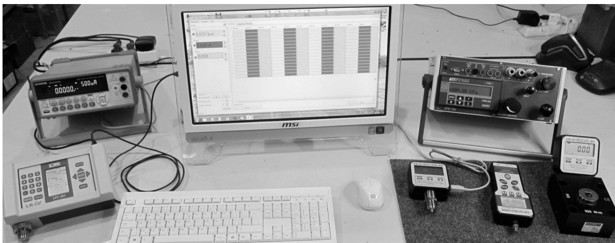
Screen of the LR-Cal/ LDM-COM software after setting the communication with three channels, in calibration table mode.
