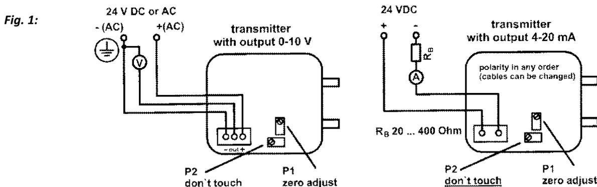
The output of transmitters with 0...10 V signal is protected against short circuit with ground and power supply. The transmitter is protected against voltage exceeding the upper limit of 30 V. The version with 4...20 mA is protected against changemengt of polarity.
