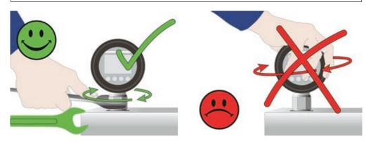
The device must only be mounted and tightened on the pressure connection using a suitable open-end wrench.
