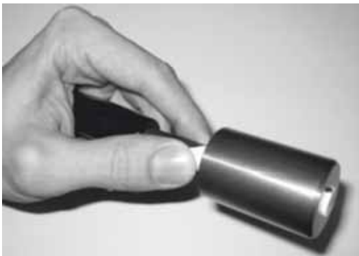
Fig. 3 Cylinder cleaning: Cleaning pin in cylinder chamber
