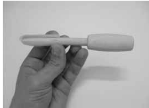
Fig. 2 Cylinder cleaning: Cleaning pin with cotton strip
