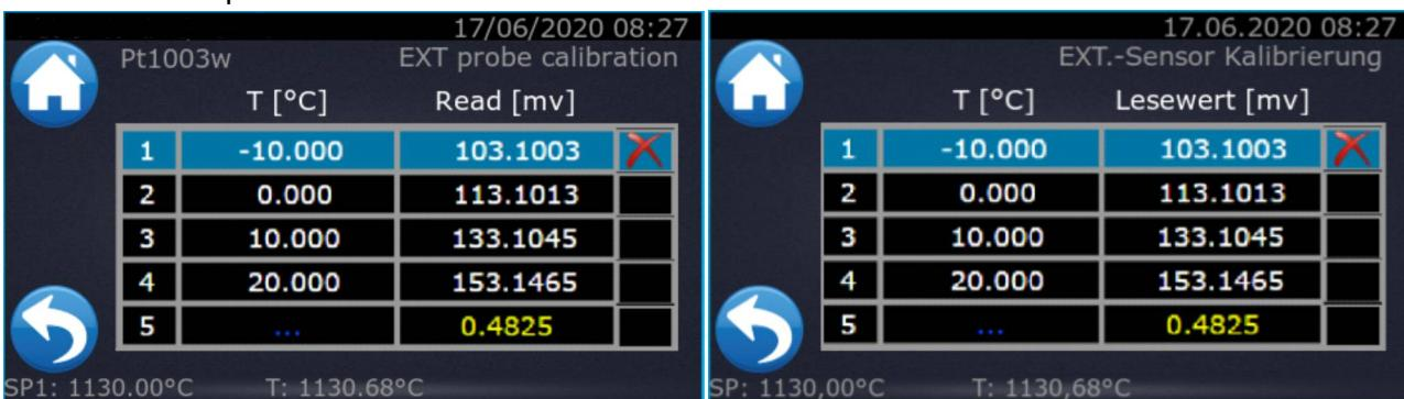
The image shows two side-by-side screenshots of a touchscreen calibration interface. Both screens display a table of calibration data with the following columns: Index (1-5), Temperature (T [°C]), and Reading (Read [mv]). A fourth column, marked with a red 'X', indicates the delete function for each row. The bottom row of the table shows the current reading for the channel.
