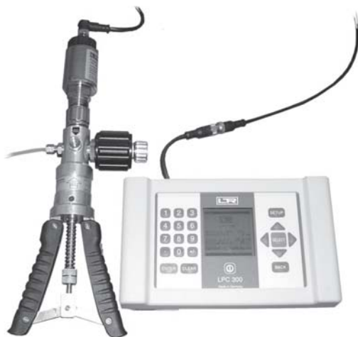
Calibration Setup with Calibration Handpump as pressure source with external connected reference sensor
