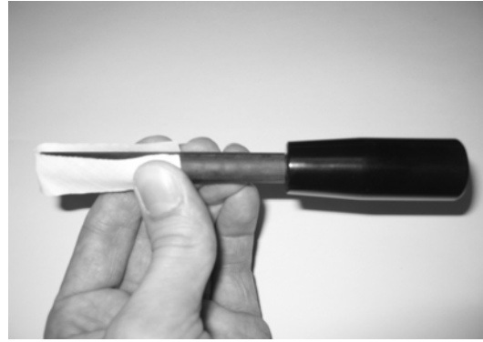
Figure 3: Cylinder cleaning: Cleaning pin with cotton strip
