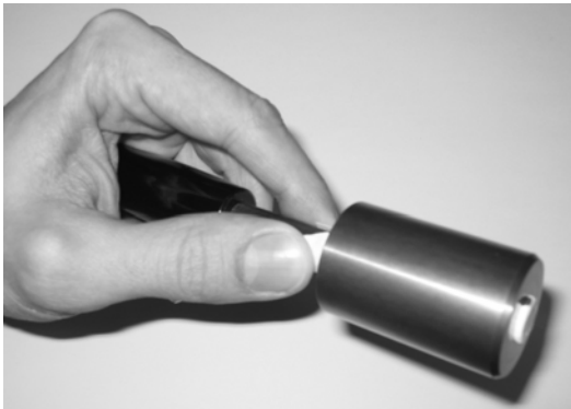
Figure 4: Cylinder cleaning: Cleaning pin in cylinder chamber
